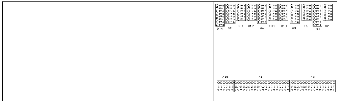
Figure 7: Position of terminal blocks with version E16E352
